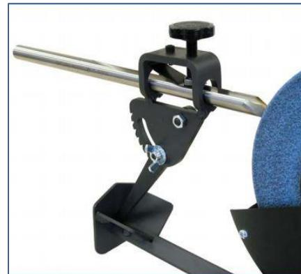
Once the tip is ground to 60 degrees, reset the tool in the Vari-Grind to again return to 2" exactly sticking out. If needed adjust the V-guide again to get back to the 60 deg grind.
