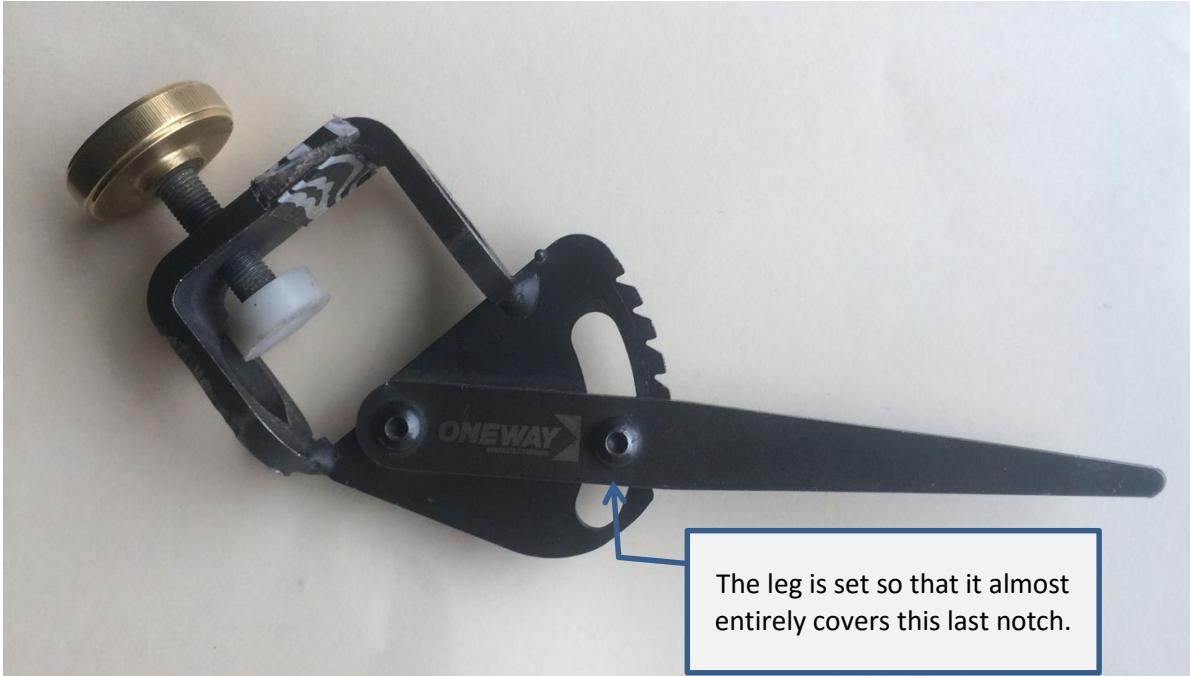
Then insert your bowl gouge so that the tip extends exactly 2" from end of the jig.
