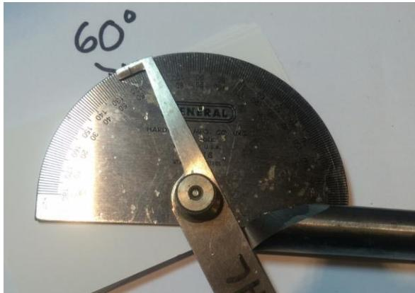
The goal for an Ellsworth Grind is to get the tip of the tool ground to an approximate angle of 60 degrees.
