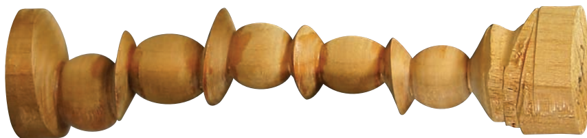
This spindle is a circular type with a twisted axis. On the right end, the axis is in the center. The left end has six axes that are placed in a circle around the center axis. After a cylinder is created on each new axis, a bead is turned. The discs connect each axis.
