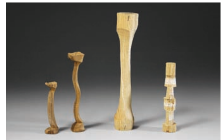
Each spindle above is an arc outcome. The third spindle from the left has twisted axes. The other three have parallel axes.
