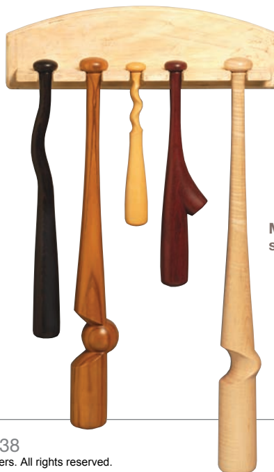
Two rectangular spindles are turned together and then rotated to create a second turning. This creates two identical spindles. The axis of split turnings can either be in the center or twisted. Split turnings create arc-type results.
