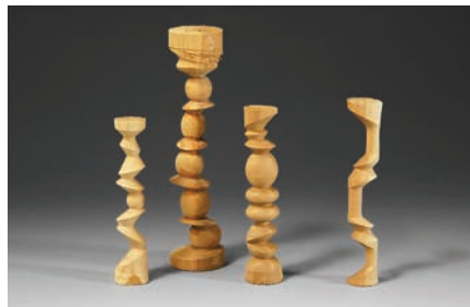
Each of the spindles above are circular outcomes. The spindle on the right was made with parallel axes; the rest have twisted axes.
