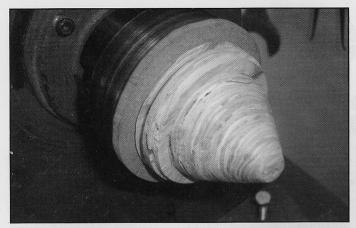
**Step 6.** Next, glue the last two pieces of the material together and mount them on a screw chuck. (*Note*: the spacer used to minimize the screw depth of the chuck.) Turn a taper that will eventually become the inside of the funnel. I try to get the total length of the funnel to be two-thirds of the depth of the domed opening in the other part of the salt shaker. I leave a flat top on the funnel of about 3/8" in diameter.
