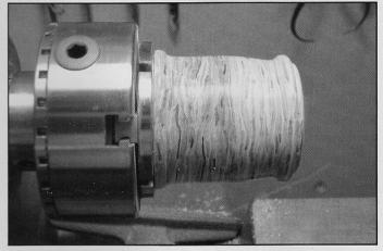
**Step 10.** Mount the shaker body on the 4-jawed chuck and do the final shaping of the outside. You can pretty much use any shape you want as long as you don't cut through to the inside.
