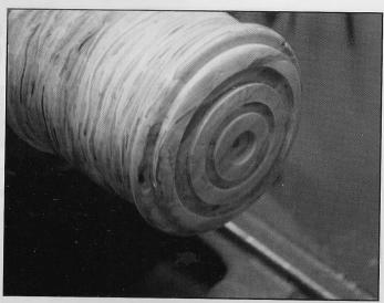
**Step 13.** Crushed turquoise and pipestone were used to inlay the grooves in my shakers, but other material would work just as well; experiment a bit. The stone is inlayed one color at a time and thin cyanoacrylate glue (CA or superglue) is used to secure the material. Sand the stone flat. Once the inlay is sanded smooth, put the final finish on the outside of the shaker.
