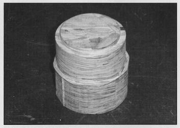
**Step 5.** Glue the two pieces together to form the body of the salt shaker.
