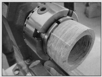
**Step 4.** Drill a hole in the middle of one of the circles of material on the drill press. This hole can be any size; it has to be just big enough to fit over the chuck jaws and 2" works well for mine. I cut the matching recess for the first tenon on the top and clean up the outside of the material.
