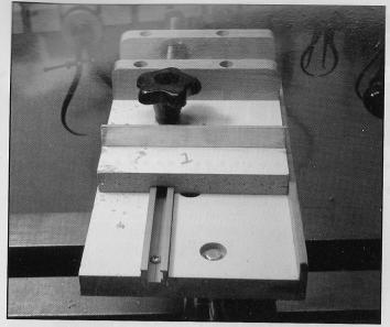
**Step 12.** Uniform spacing of the grooves makes a big difference in how the decoration appears, so I use this jig to ensure that the grooves are even. At sixteen threads to the inch, each complete turn of the handle gives me 1/16". With the jig, I can keep the grooves even across the top. I put the grooves 3/16" apart which I've found gives the top a nice appearance. However, you can use a parting tool to accomplish the same thing; you just have to be a bit more careful.
