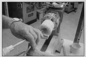
**Step 8.** Insert the funnel into the main body and begin to hollow out the inside of the funnel. This requires a very snug
