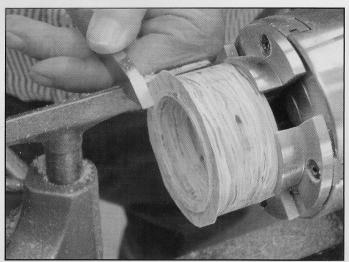
**Step 3.** Cut a tenon on the side of the dome to align the next piece of material.
