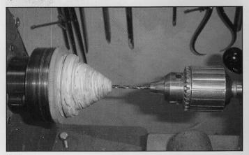
**Step 7.** Drill a 1/8" hole in the top of the funnel. This is done now so the hole will be in the center of the funnel. I also create a tenon on the bottom of the funnel that will mate snugly in the main body of the shaker. This last step is critical to the success of the next step.
