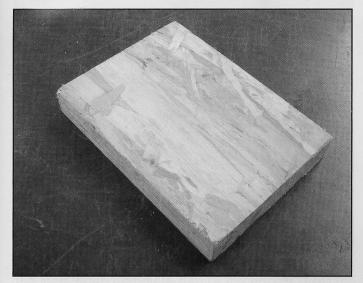
**Step 1.** I started with construction material obtained by dumpster diving at a nearby truss manufacturer. The use of construction grade chipboard rather than solid wood is for two reasons. First, it is very stable and does not move or distort. Second, and the main reason, it is very difficult to ascertain the glue lines once the blank has been glued together.
