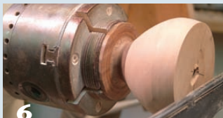
6 Reverse the bowl into a four-jaw chuck using the tenon formed on the base.
