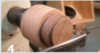
4 With the bowl blank mounted on a screw chuck, turn the bowl and base sections round, cut a tenon for remounting the blank, and mark the center of the tenon.
