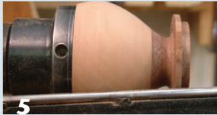
5 Begin to shape the bowl and base, leaving the tenon intact for remounting.
