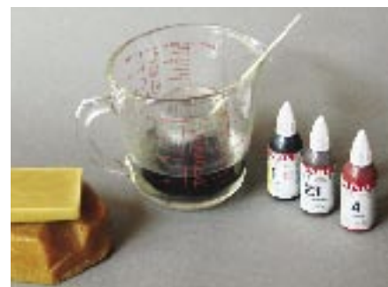
You can easily tint small batches of wax by first melting wax shavings in a bath of hot water, as shown above. Then, blend in tinting bases to add color before cooling the mixture. Mixol, a universal tinting base manufactured in Germany, is available in 20ml bottles from Woodcraft and other woodturning suppliers.
