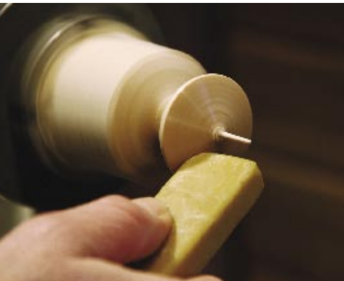
Apply stick wax to pieces while still mounted on the lathe. Bill Hunter softens the sheen of a cocobolo piece with 4/0 steel wool.
